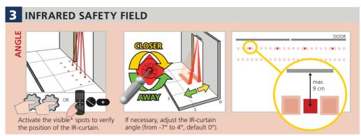
\* Visibility depends on external conditions. When spots are not visible, use the Spotfinder to locate the curtains.
