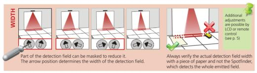
The size of the detection field varies according to the mounting height and the settings of the sensor.
